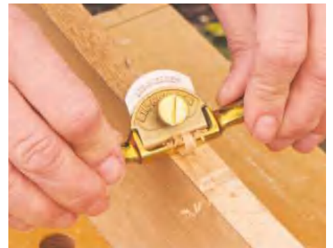
STEP 6. Clean up the curve with a spokeshave. Alternatively, use a sanding drum fitted in a drill stand if you prefer
